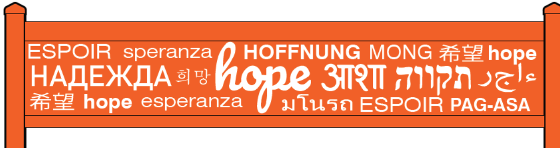
BOARDING ISLAND RAILING STEEL TUBE FRAME/LASER CUT PANEL
