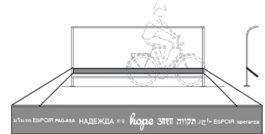
BIKE LEANING RAIL TUBE/LASER CUT PANEL
